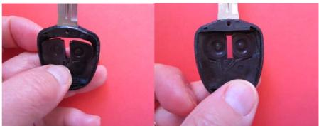
New Silicone buttons will be fitted from inside of the remote. Simply press fit silicone buttons in respective button holes and groove inside plastic shell.
