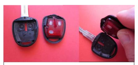
Once your silicone buttons are fitted in, place electronic board back in remote, cover it with bottom part of the shell and screw it together. **No reprogramming is need it** as remote will work straight away.
